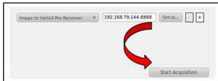
FIGURE 1.13 Initiating remote memory acquisition
