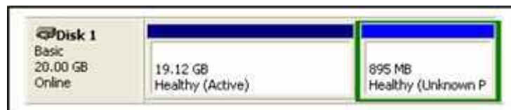
FIGURE 1.62 Identifying the subject system's drive in the Disk Management snap-in
