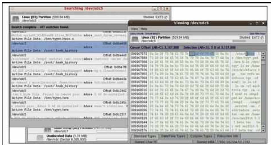
FIGURE 3.18 Keyword searching for the string “adore” using SMART forensic tool 14
