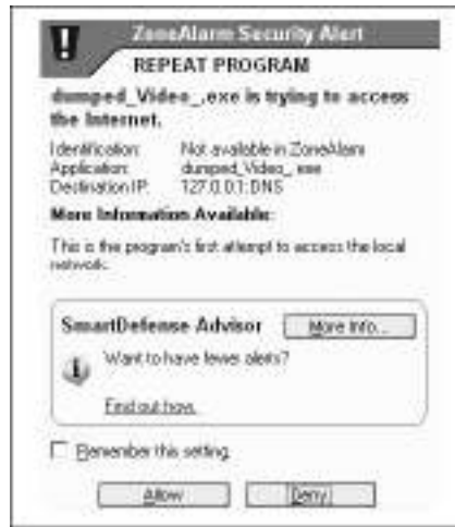
Figure 9.46 The New Executable “Phoning Home” to Resolve a Domain Name
