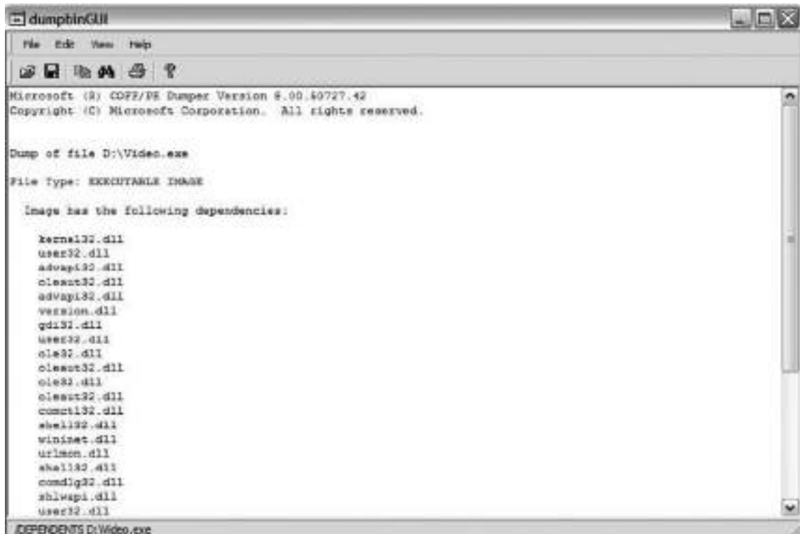
Figure 7.35 Inspecting video.exe with DumbinGUI
