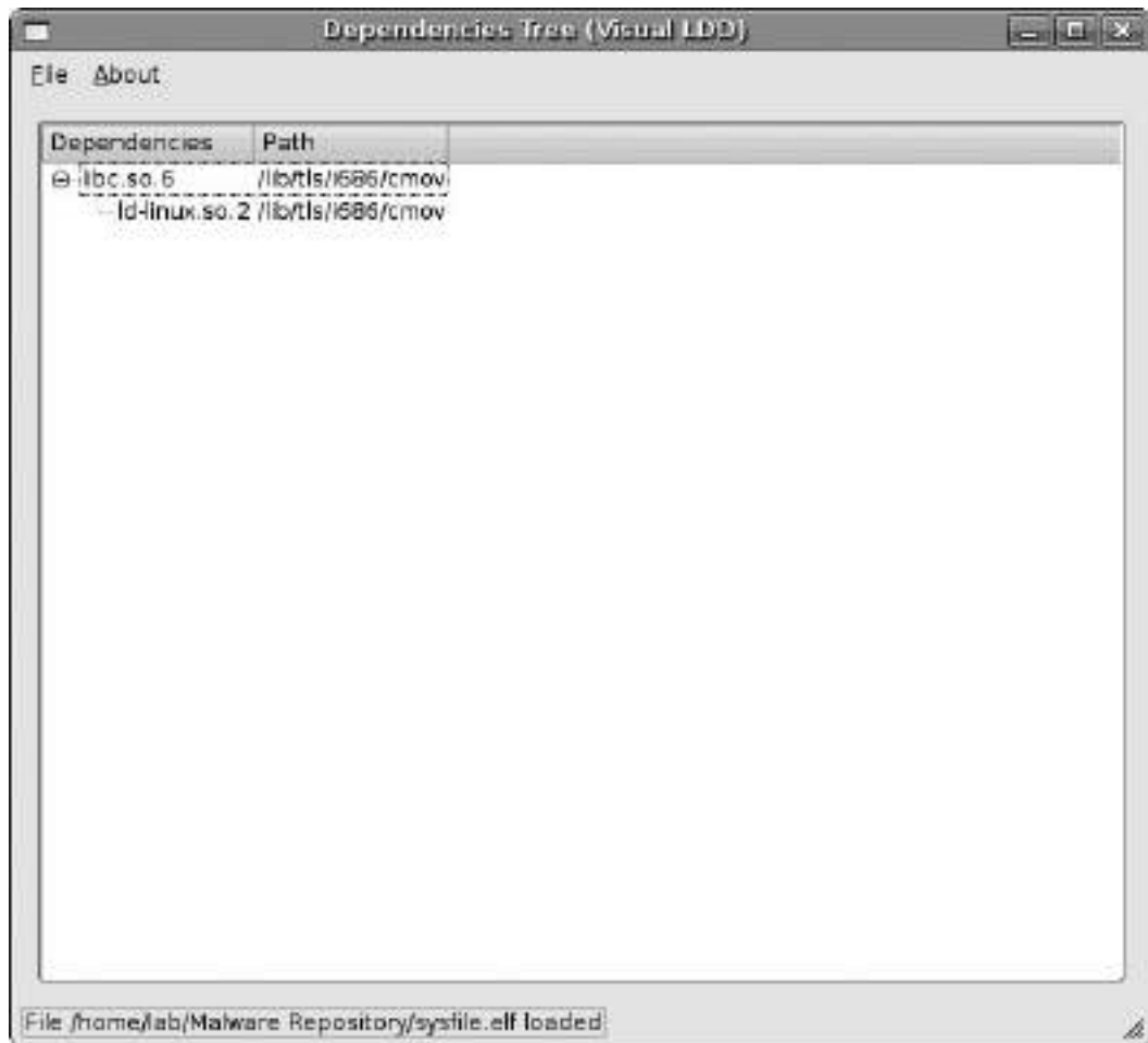
Figure 8.44 Inspecting sysfile with Visual Dependency Walker
