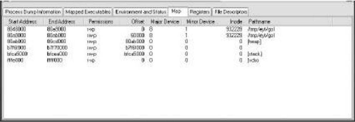
Figure 3.32 Memory Parser Displaying Memory Mappings for the “gol” Process
