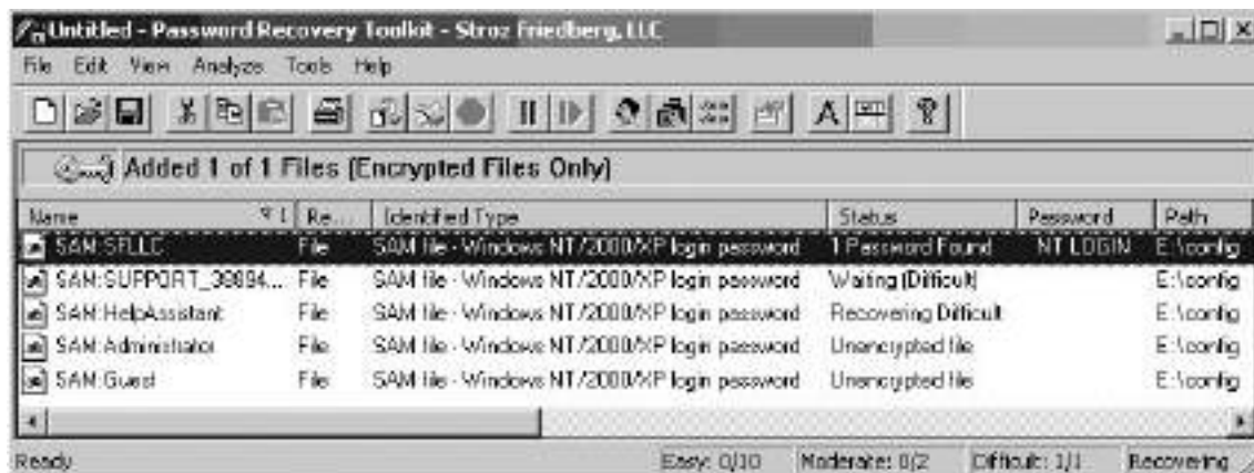
Figure 4.13 Password Guessing Using the Password Recovery Toolkit
