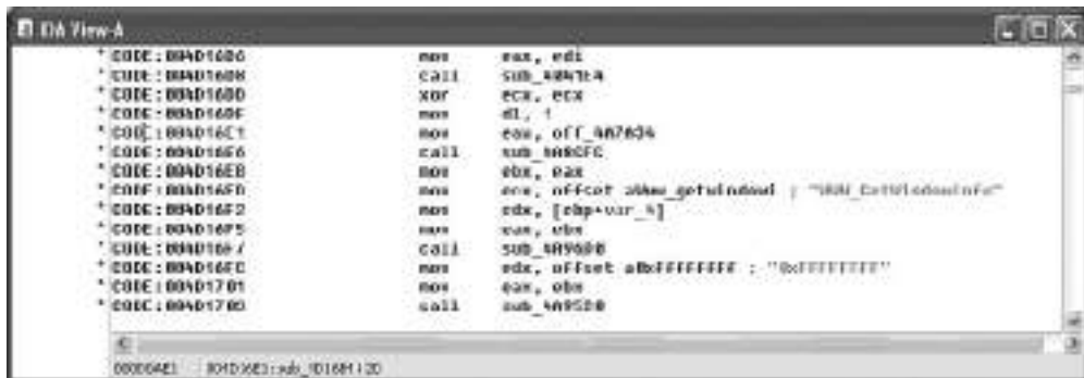
Figure 9.50 Discovering the WWW_GetWindowInfo Command in IDA Pro
